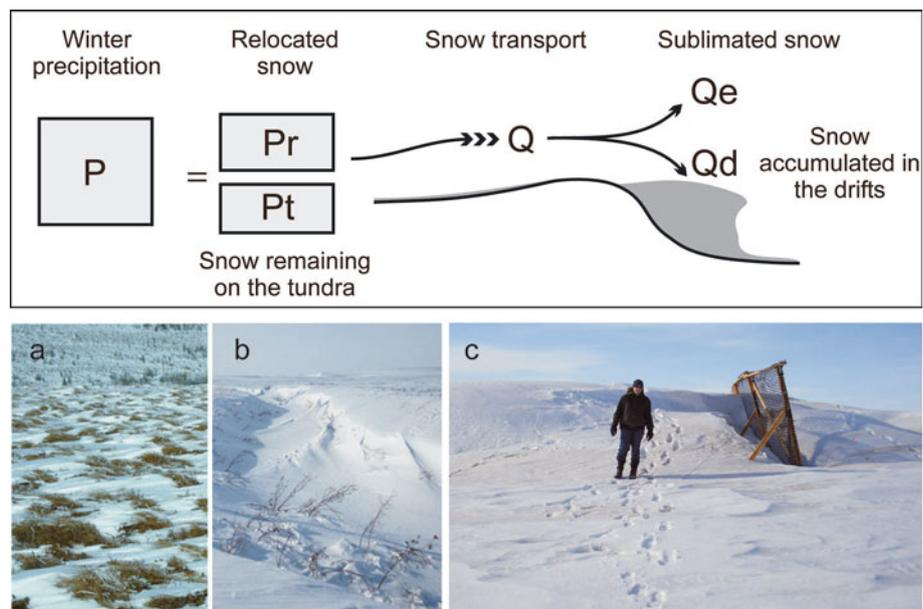
**Fig. 1.** (a) Benson's (1982) partitioning of the wind-blown flux of snow. (b) Tundra tussocks have trapped  $P_r$ . (c) A gully and (d) a snow fence have trapped  $Q_d$ . The gully is not full, but the fence, with the wind blowing from right to left, appears to have reached its equilibrium profile.
