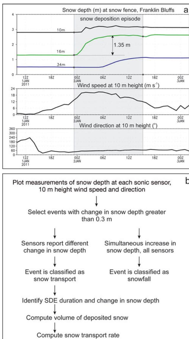
**Fig. 4.** (a) Sample sonic sounder and weather records and (b) the rubric used to identify snow deposition events from this and other records.
