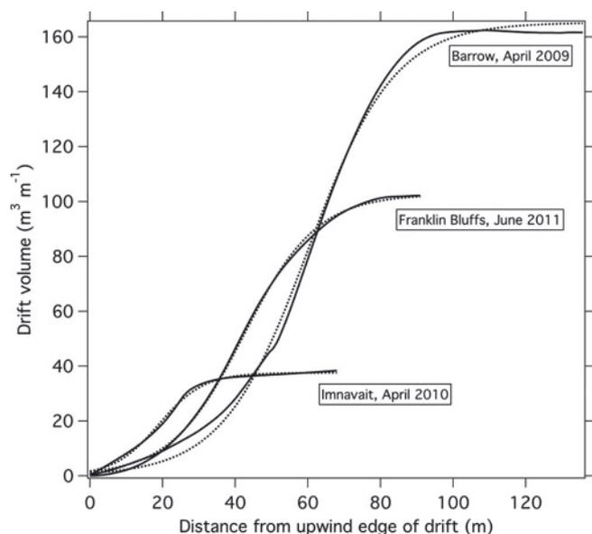
**Fig. 7.** Surveyed cumulative drift volume curves (solid) compared with the results of Eqn (3) (dotted). In those cases where a deep v-shaped moat was present at the fence, a small jog appears in the measured curve (Barrow, April 2009 at  $x = 50$  m). Fitting parameters ( $V_{total}$ ,  $d$  and  $s$ ) are given in Table 4.
