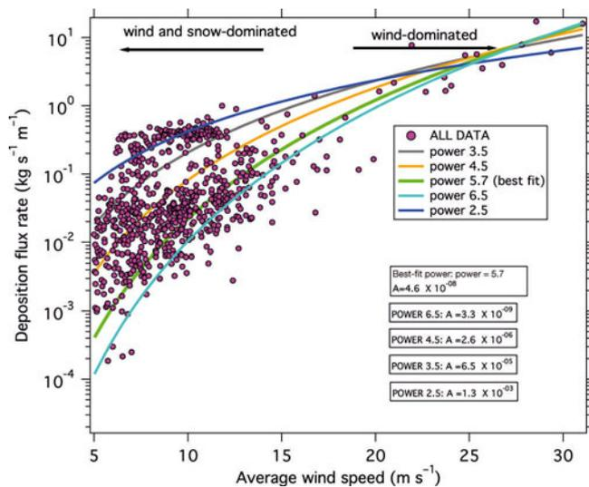
**Fig. 12.** All blowing-snow flux data from Figure 10, including data from this study, with a series of power curves fit to the data. Upper and lower bounding curves are listed in Eqns (5) and (6) and are suggested as bounding curves for the data.
