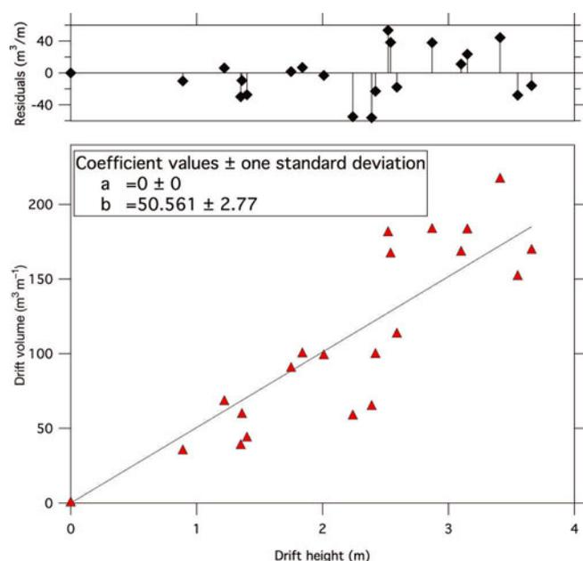
**Fig. 9.** Drift volume as a function of drift height, in this case as indicated by averaging the values from three sonic sounders taken at the time of each profile survey. Data are from all surveys at all fences and the regression has been forced through (0,0). The residuals are shown at the top.
