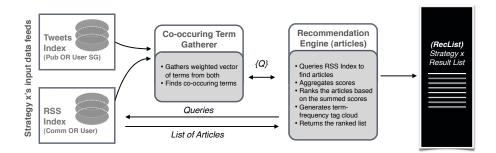
Fig. 2. Generating results for a given strategy. System mines a specified RSS and Twitter source and uses the co-occuring technique described to generate a set of results, which will be interleaved with other sets to produce the final list shown to users.
